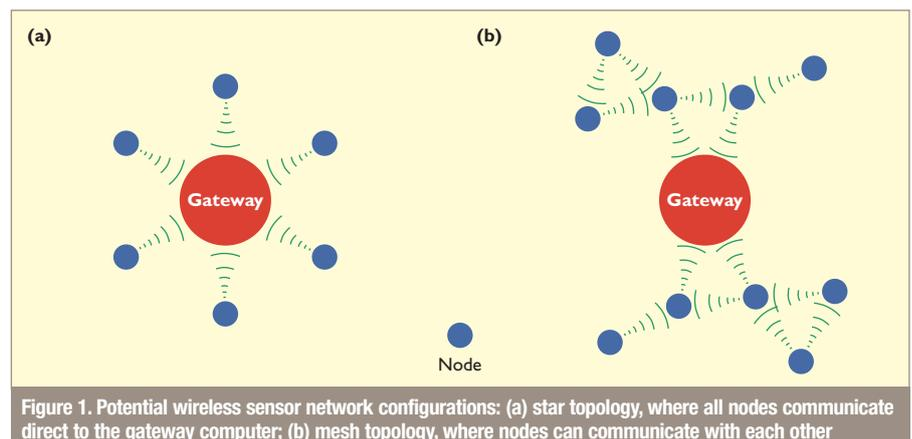
Figure 1. Potential wireless sensor network configurations: (a) star topology, where all nodes communicate direct to the gateway computer; (b) mesh topology, where nodes can communicate with each other
