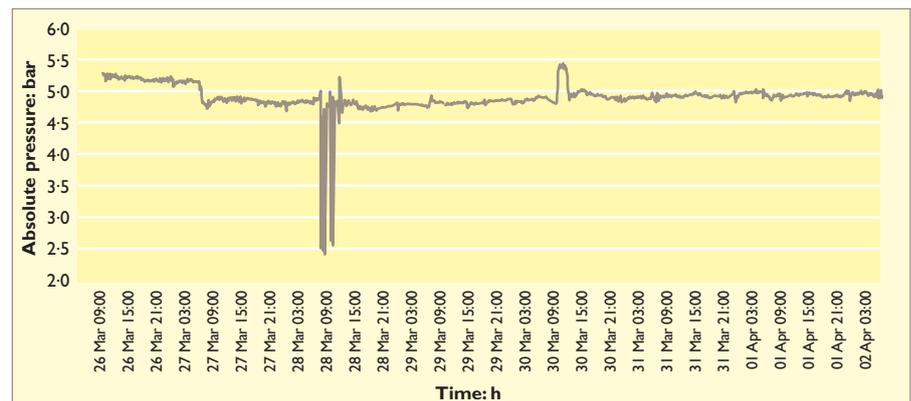
Figure 11. Mains water pipe pressure measured continuously at 200 samples per second over a period of 1 week revealed a potentially damaging pressure surge
