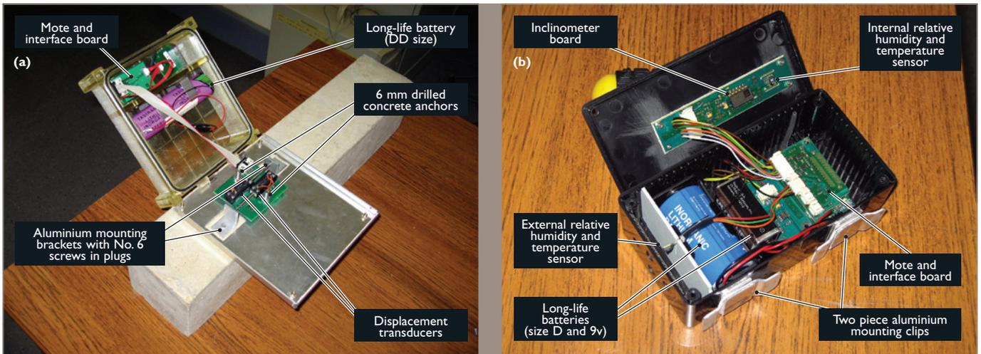
Figure 4. Ferriby Road Bridge sensors: (a) displacement transducer to measure crack widths as well as temperature and relative humidity; (b) inclinometers installed on elastomeric bearings
