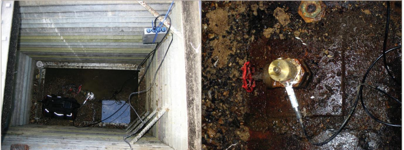
Figure 8. Water-pressure measurement node: (a) pressure sensor and node viewed down manhole; (b) close-up of pressure sensor
