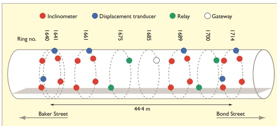
Figure 7. The London Underground wireless sensor network was arranged over five separate tunnel rings – relay nodes are used to transmit data to the gateway
