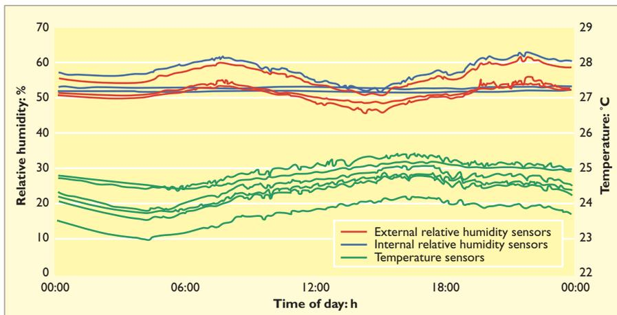
Figure 10. Relative humidity changes in London Underground are less consistent than temperature changes and appear to be linked to the humidity in the stations and outside
