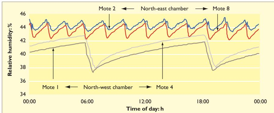
Figure 9. Relative humidity in the north-west Humber Bridge anchorage chamber varies far more than that of the north-east chamber, yet the dehumidifier uses less energy as it powers on less often
