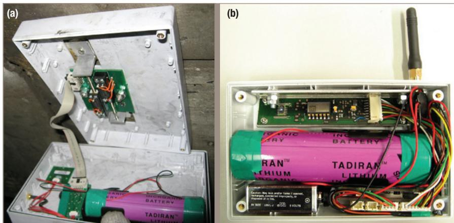
Figure 6. London Underground sensor nodes, which had to protrude no more than 35 mm from the tunnel wall: (a) displacement transducer to measure movement at tunnel crown and crack widths; (b) inclinometers installed on precast concrete tunnel lining panels
